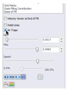
Step 3: Look at the purples spheres. They indicate locations where air is likely to get trapped. The more frequently these spheres appear, the more air will get trapped due to the design of the part.
